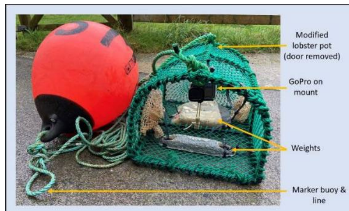
Figure 4.4 GoPro fixed in modified lobster pot.
