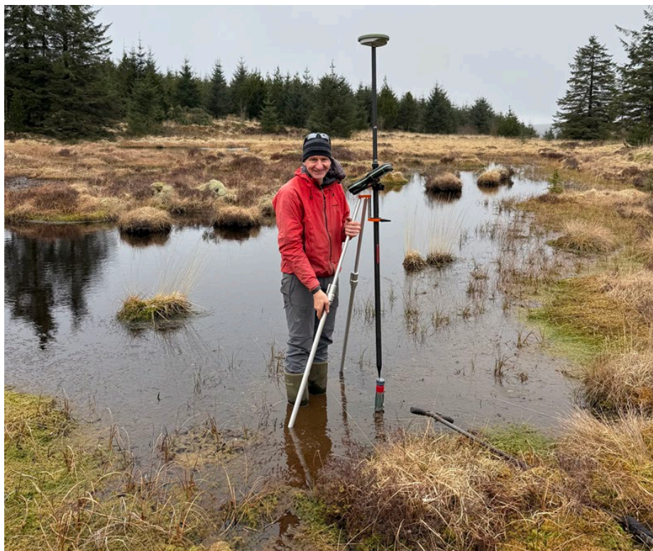
Figure 19. A newly installed dipwell being surveyed into OS and height datum by Dr Rob Low, consulting hydrologist to NPAP, at Cors Gerwyn, Tywi Forest.
