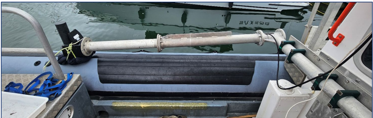
Figure 9 – Extended survey pole in recovered position. Note that it now puts the sonar head in line with the engine hatch (left of photo).
