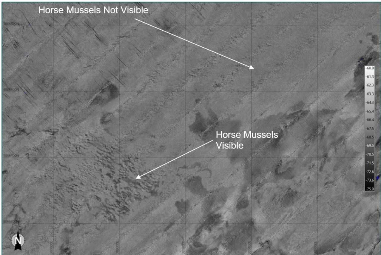
Figure 14 – Backscatter data over the same area as Figure 13. Mussel extent in the SE is clearly visible, however the northerly portions cannot be delineated. Coloured by intensity value (dB).
