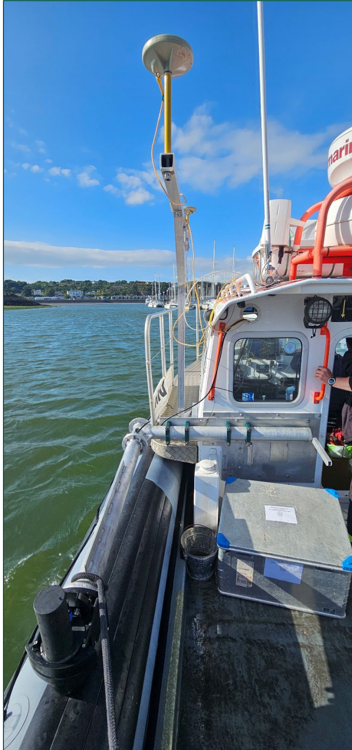
Figure 3 – Survey pole and antenna T-Bar in recovered and stowed position
