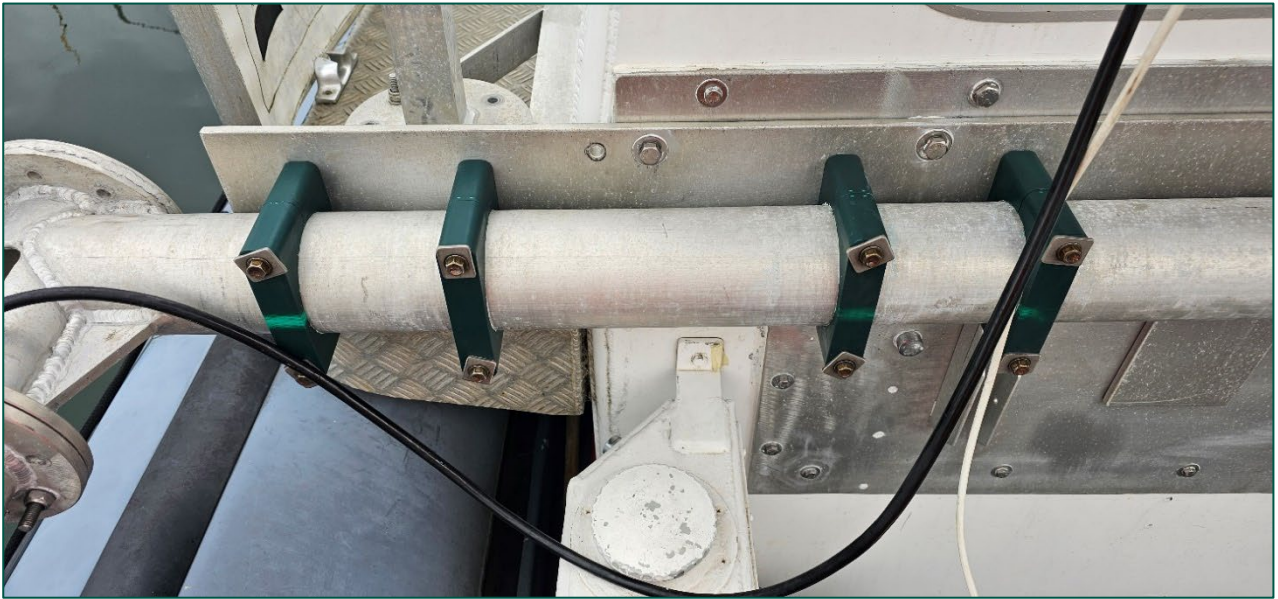
Figure 10 – The Stauff™ clamps used to hold the survey pole in position. Note the discoloured stress marks, particularly on the outer clamp on the left of the photo.
