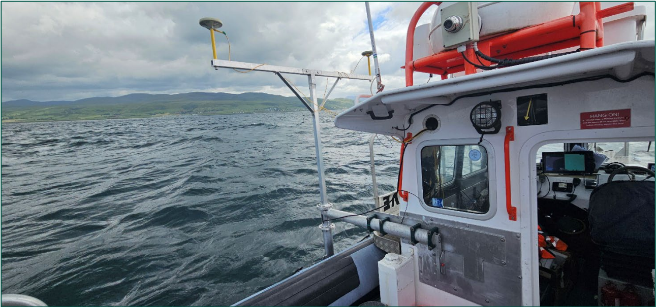
Figure 4 – Survey pole and T-Bar in deployed position
