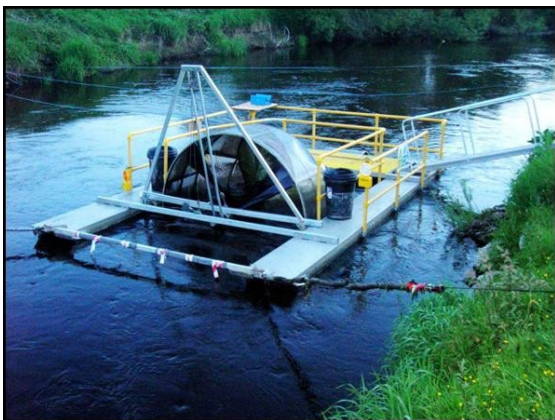
Rotary Screw Trap used to capture smolts on the lower Dee
