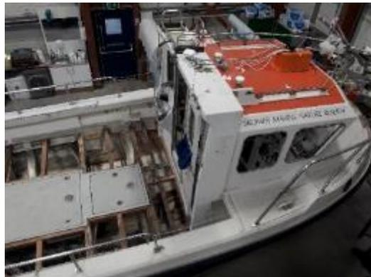
*Skalmey* has now served the MCZ (and MNR before that) for 27 years and so a thorough “health check” seemed in order. After a detailed professional survey of the hull and the equipment of the boat considerable remedial action was recommended. This included replacement of the deck and deck beams (now distinctly soggy and saggy in parts), replacement of windows (dribbly), replacement of the fuel tanks (crusty) and thorough overhaul of the engine (wheezy).
