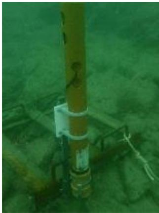
The greatly reduced seabed frame at Thorn Rock functioned perfectly well as a mount for the sediment trap (Newman Poot Collector – pat. pending) with new mounting arrangements made from recycled parts from the seabed settlement plate studies carried out in previous years.
