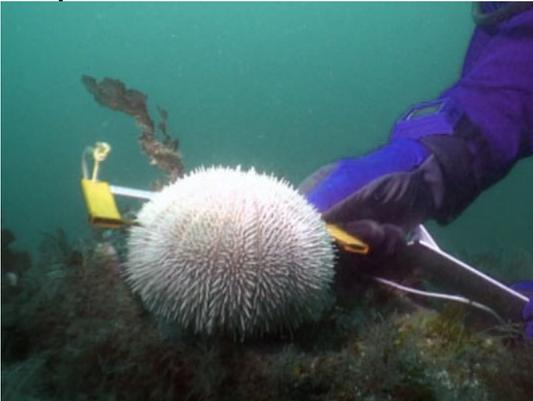
The value recorded on the dividers is the tangential meeting point of the rulers with the urchin. The trigonometry required to determine the diameter of the urchin from the value measured off the dividers (which should be equal on both rulers) is illustrated.
