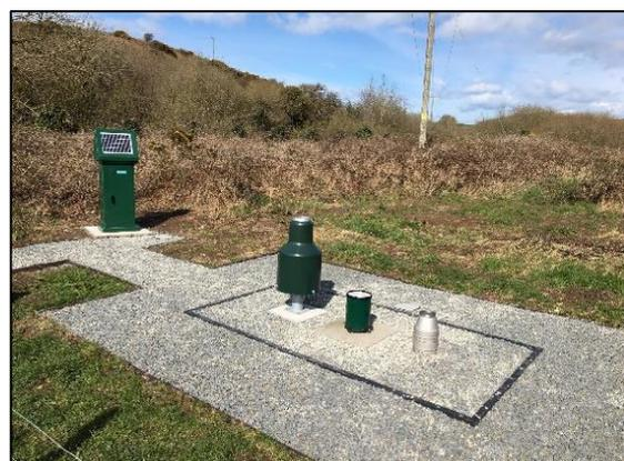
**Figure 6: A rain gauge in St Davids, Pembrokeshire which has been telemetered to support the development of improved flood forecasting in the area.**
