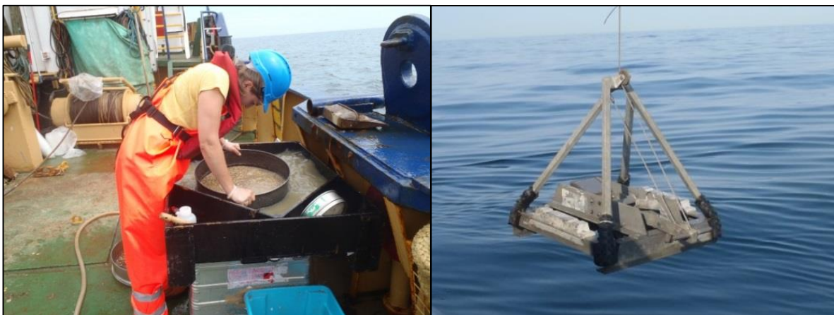
Figure 2. Sieving a grab sample on board (left); deploying a Hamon grab (right). Images © APEM Ltd
