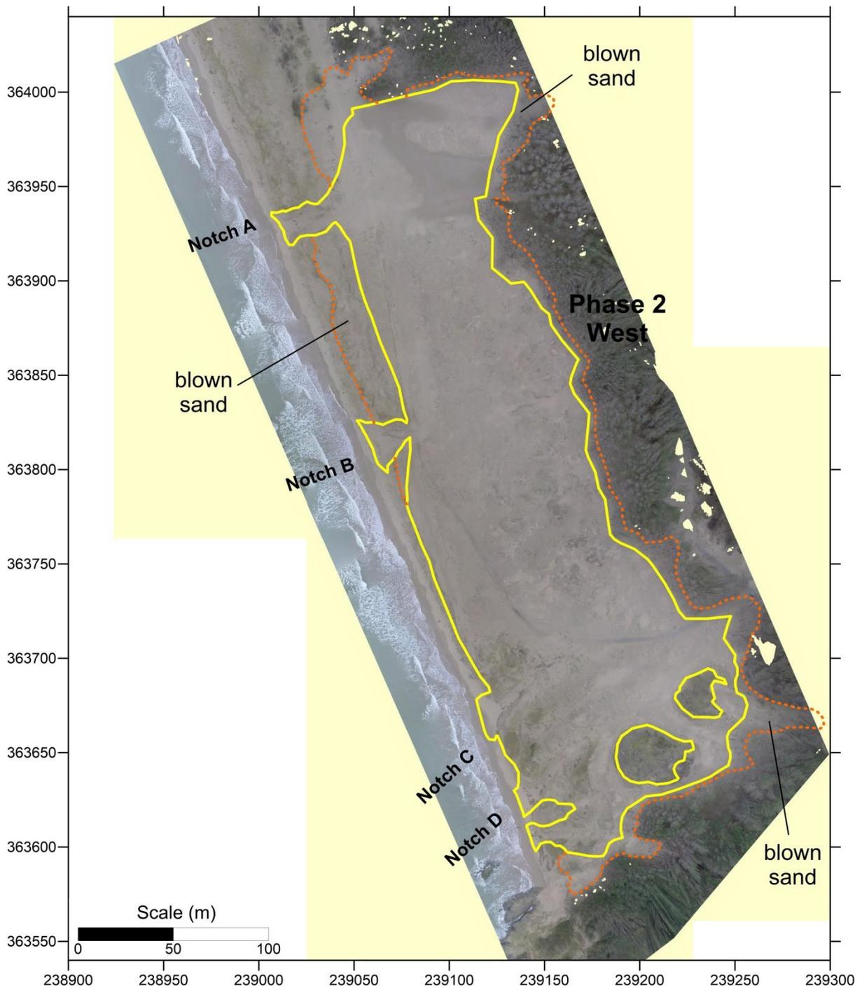
**Figure 63.** UAV aerial imagery flown January 2016 showing the extent of bare sand on the Phase 2 West works at Newborough, undertaken December 2014 to March 2015. The yellow lines indicate the bare sand areas created in December 2014 to March 2015, the orange dashed lines the areas of blown sand outside the works areas by January 2016 (note that some areas are estimated due to incomplete UAV coverage)
