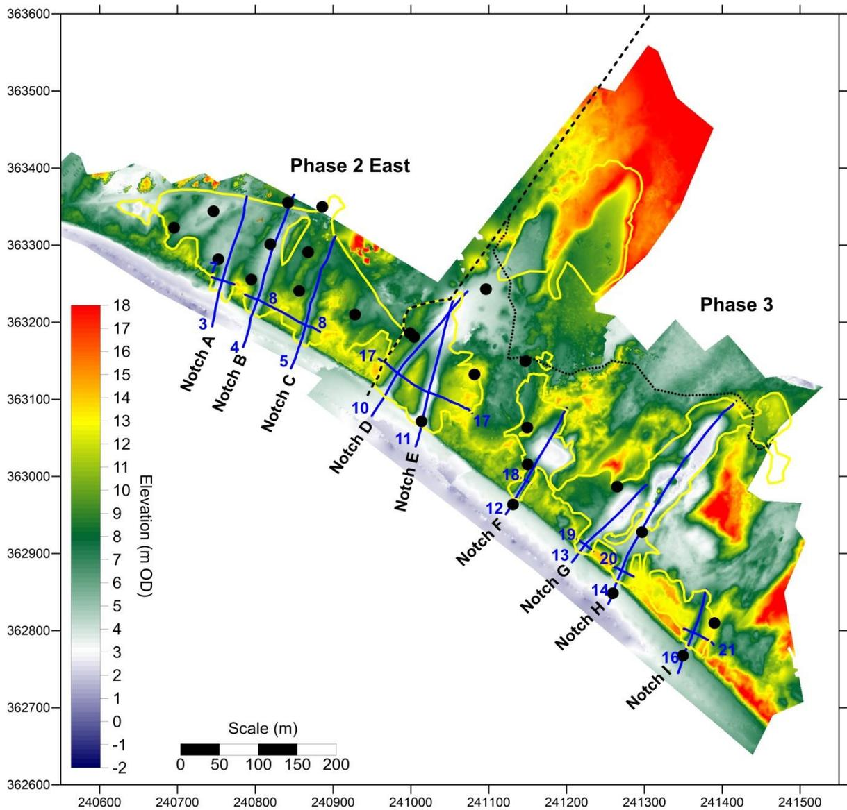
**Figure 77.** DEM of Newborough Warren Phase 2 and 3 areas, based a UAV survey in January 2016, after the rejuvenation works. The calibration points used by the survey company to correct the elevations are shown as black dots
