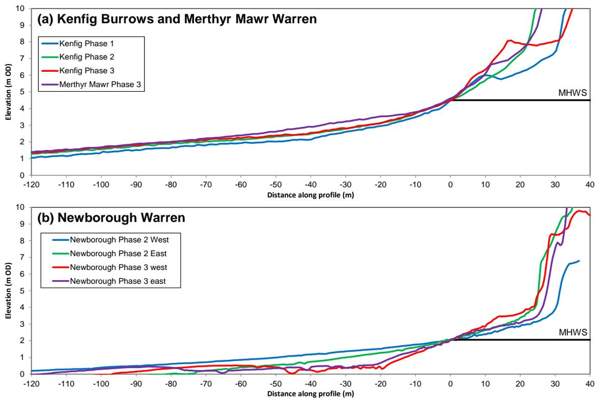
**Figure 88.** Comparison of topographic profiles across the beach at (a) Kenfig Burrows and Merthyr Mawr Warren and (b) Newborough. Elevations taken from LiDAR surveys in 2014 and 2015. The horizontal red lines indicate the levels of MHWS and MLWS.
