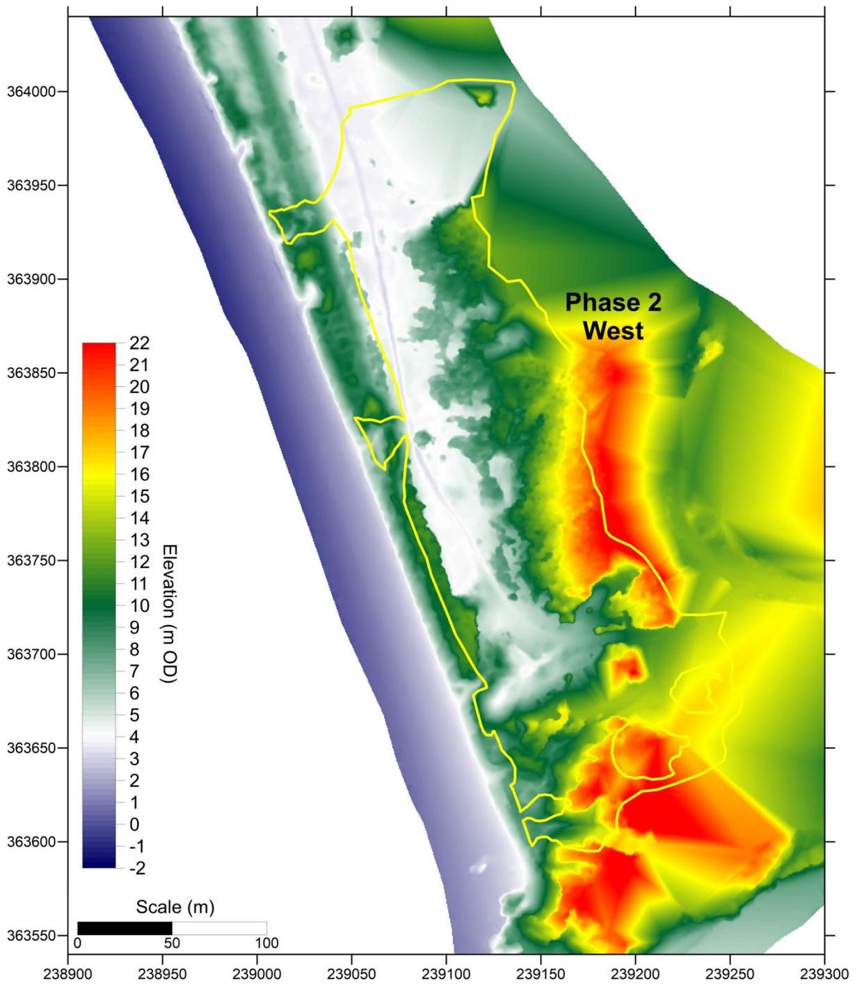
**Figure 65.** DEM of Newborough Phase 2 West area, from a UAV survey in June 2013, before the rejuvenation works
