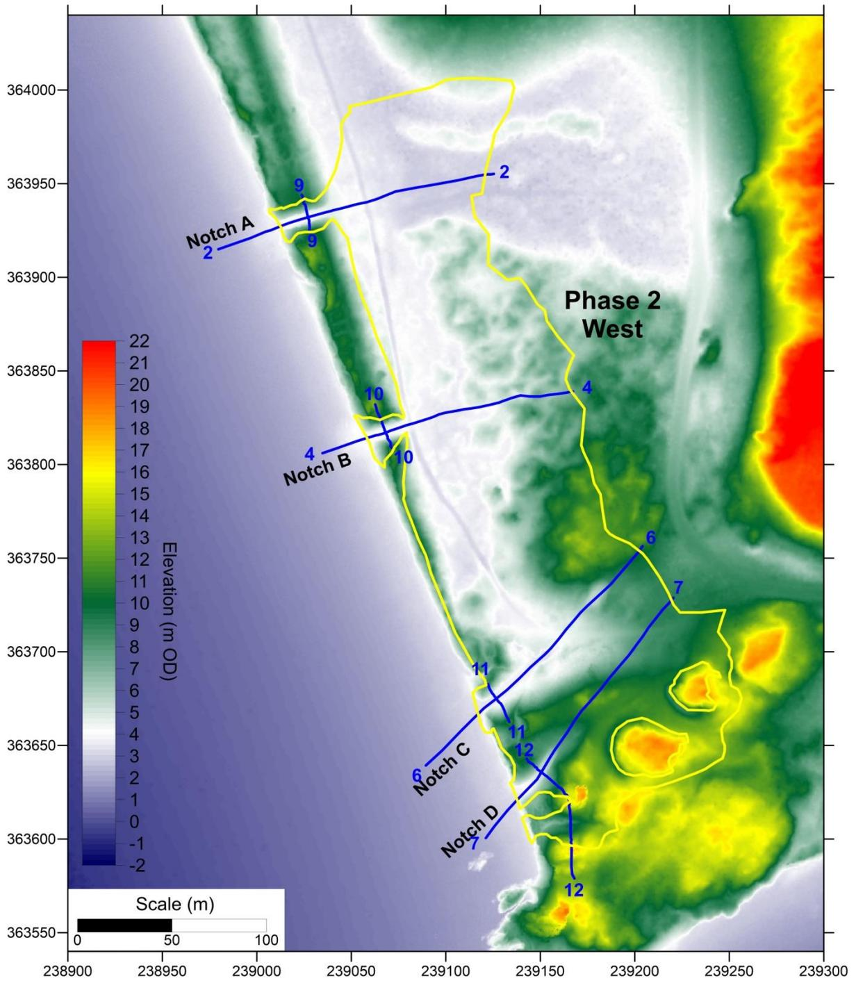
**Figure 66.** Filtered DEM of Newborough Warren Phase 2 West area, from an aerial LiDAR survey on 9 April 2014, after the rejuvenation works
