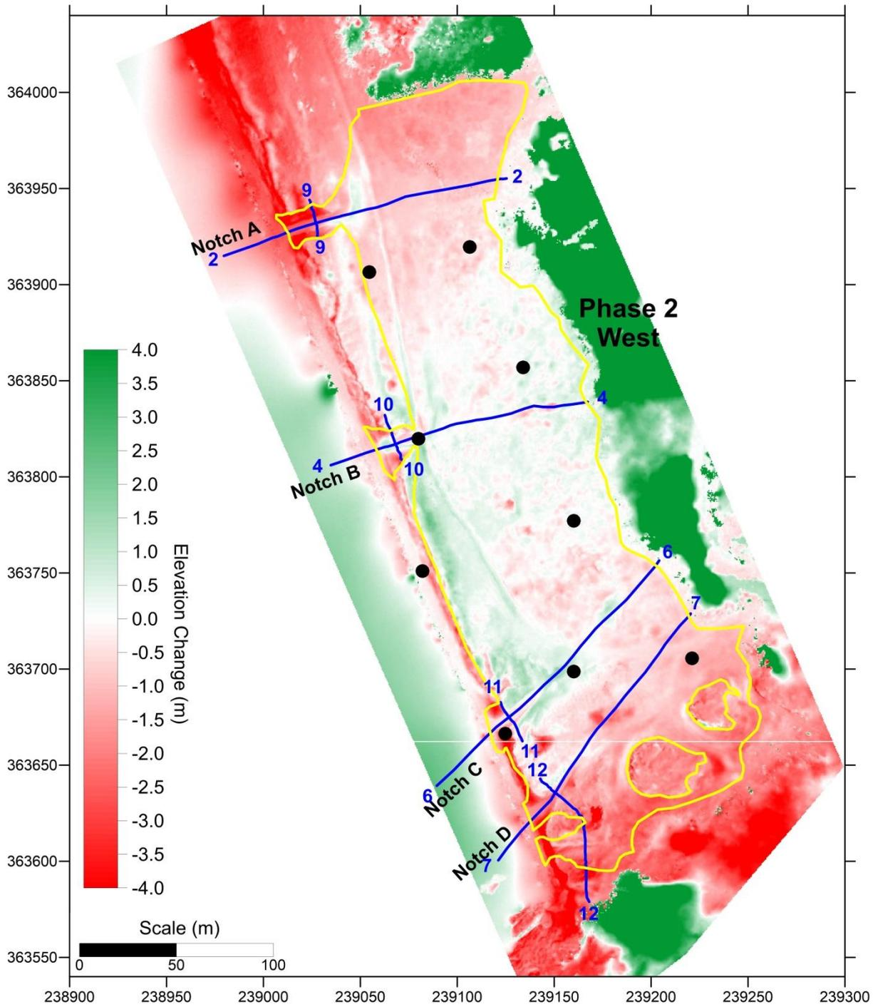
**Figure 68.** Difference in elevation between 2014 aerial LiDAR survey and 2016 UAV survey DEMs. The 2016 UAV DEM is unreliable beyond the limits of the works areas. The calibration points used by the survey company to correct the elevations are shown as black dots
