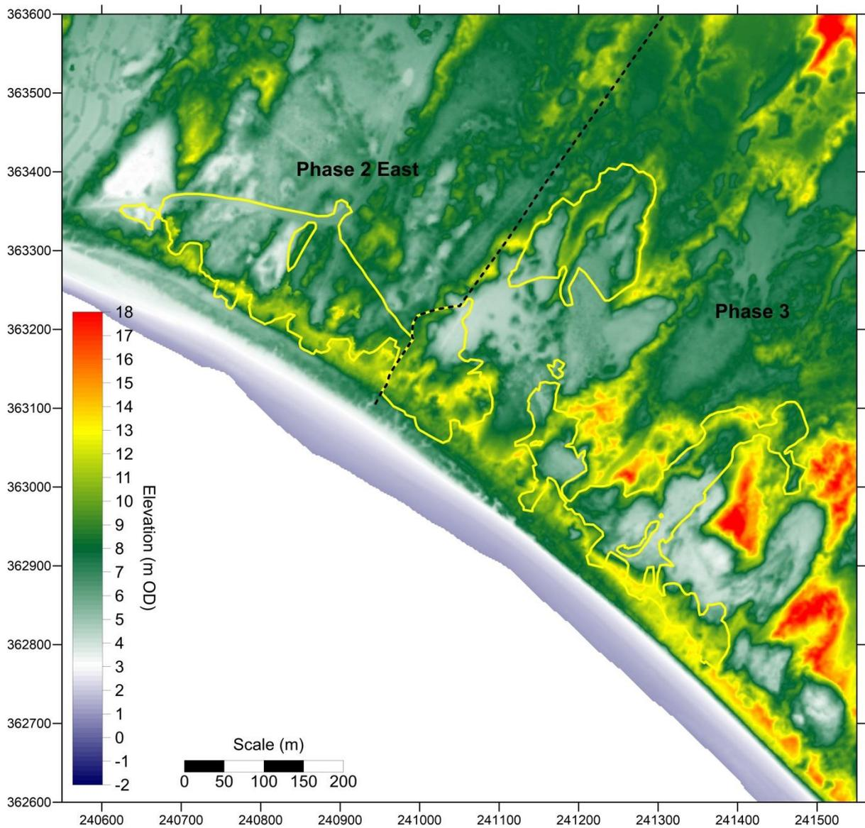
**Figure 74.** Filtered DEM of Newborough Phase 2 East and Phase 3 areas, based on an aerial LiDAR survey on 12 May 2009, before the rejuvenation works
