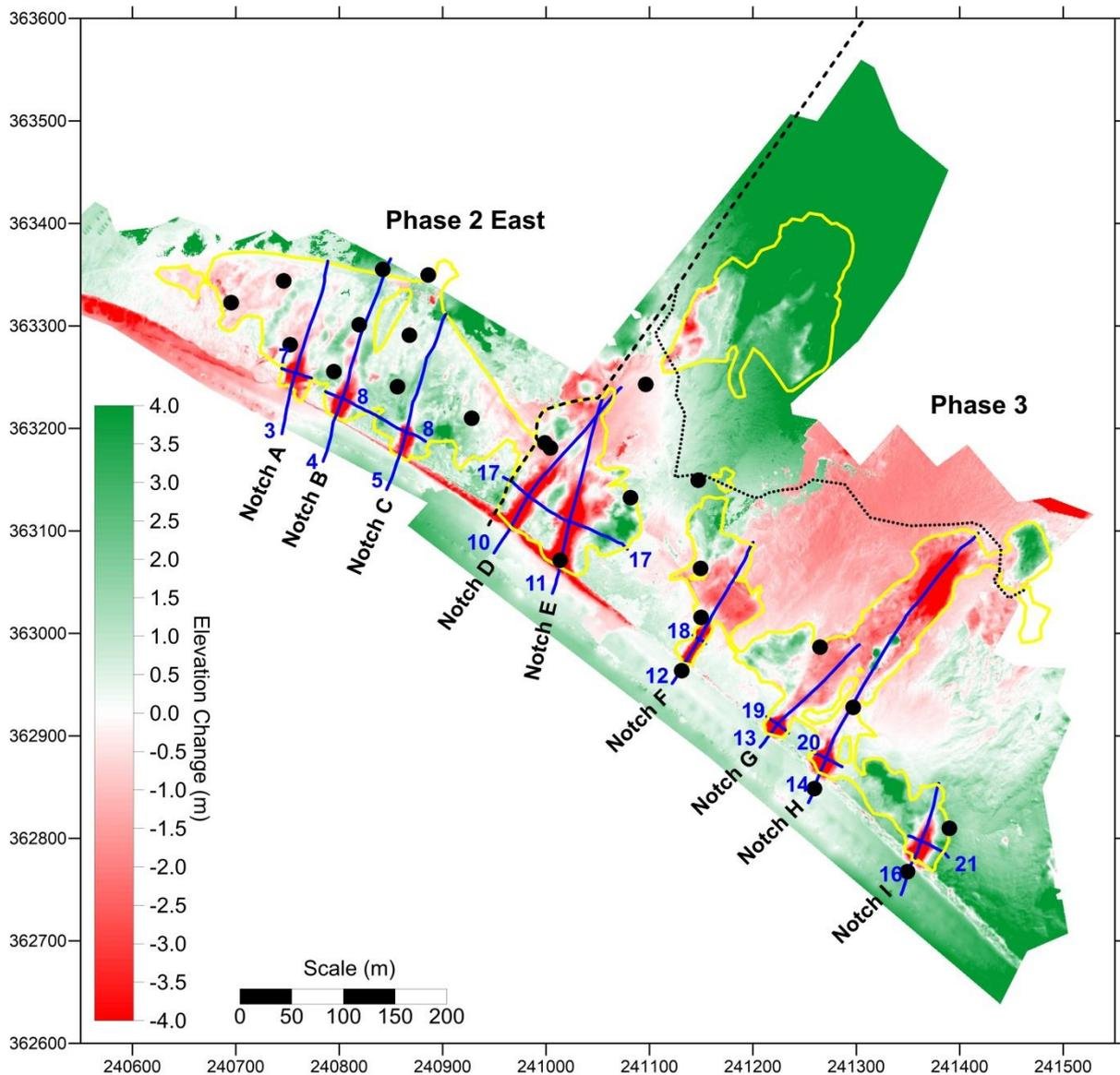
**Figure 78.** Difference in elevation between 2014 aerial LiDAR survey and 2016 UAV DEMs. The 2016 UAV DEM is unreliable beyond the limits of the works areas (in particular to the north of Phase 3, leading to apparent accretion of well-vegetated dunes), and the ‘step’ in elevation running SW-NE through the Phase 3 area. The calibration points used by the survey company to correct the elevations are shown as black dots
