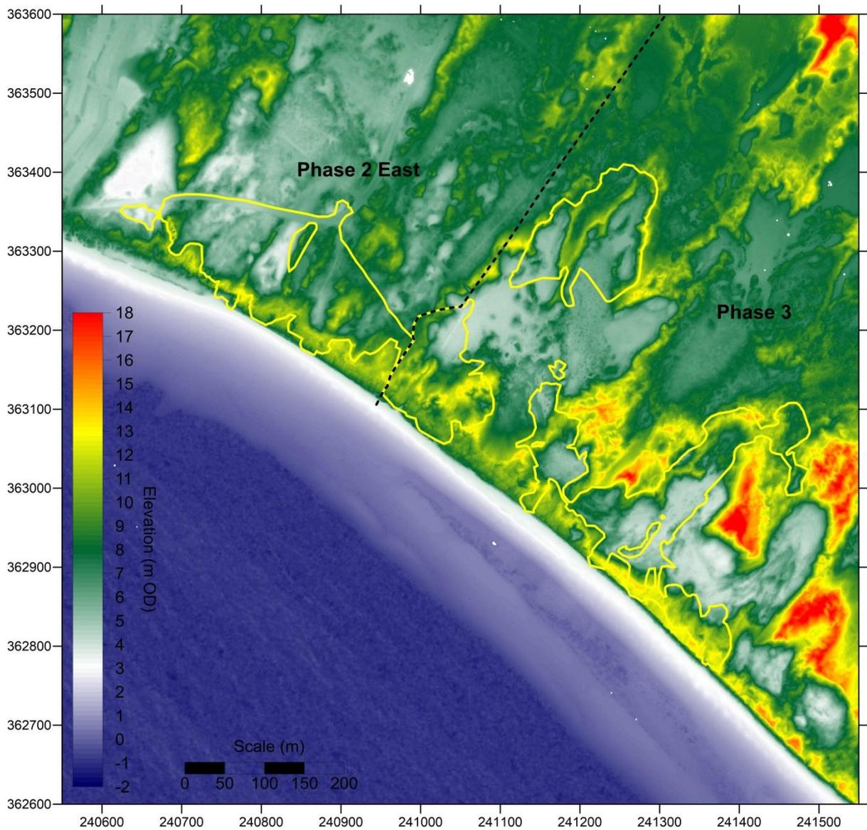
**Figure 75.** Unfiltered DEM of Newborough Phase 2 East and Phase 3 areas, based on an aerial LiDAR survey on 9 April 2014, before the rejuvenation works
