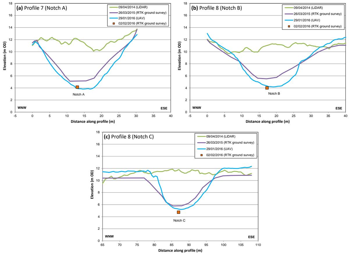
**Figure 80.** Topographic profiles across the notches in the Newborough Phase 2 East area. Elevations pre-works are shown from the aerial LiDAR survey flown 09/04/2014. Elevations post-works are shown from the subsequent ground RTK survey on 26/03/2015 and the UAV survey on 29/01/2016. Cross-profiles were not measured during the ground RTK survey on 02/02/2016, but the position and elevation at which the axial profile crosses the cross-profile is indicated with an orange square
