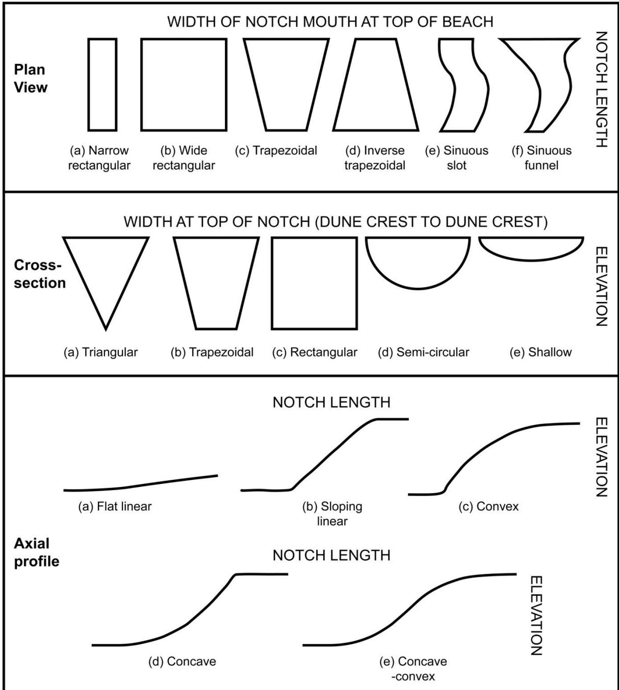
**Figure 95.** Conceptual diagram of different notch morphology, in terms of plan view, cross-section, and long section
