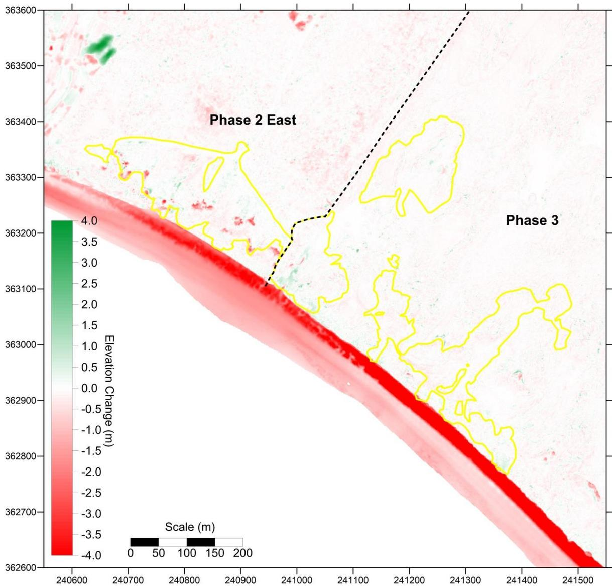
**Figure 76.** Difference in elevation between 2009 and 2014 aerial LiDAR DEMs. Very little sediment from frontal dune erosion appears to have moved inland to the dunefield
