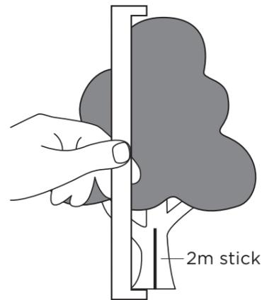
Figure 3. Lining up the hypsometer scale for measurement.
