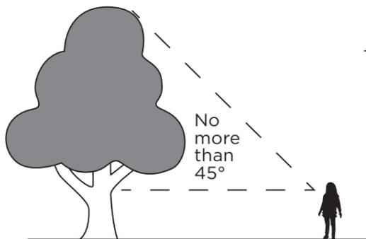
Figure 2. Correct distance from tree for hypsometer measurement.
