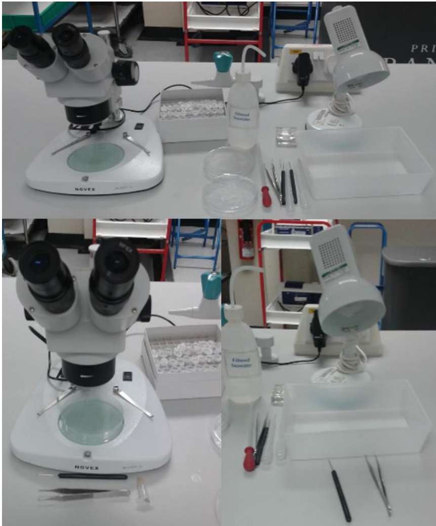
Figure 9. The total set up for analysis showing the directing microscope, Eppendorf tubes, filtered sea water, container for sorting through the samples, Petri dishes, pipettes and tweezers.
