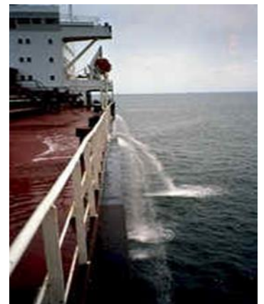
Figure 5. Ballast water being pumped from a large vessel. Source: massbay.mit.edu
