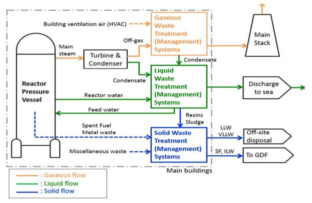
Figure 8.1: Diagram of gaseous, liquid and solid waste arisings within the UK ABWR (from Hitachi-GE's Summary of the Generic Environmental Permit Applications GA91-9901-0019-00001 Revision H).
