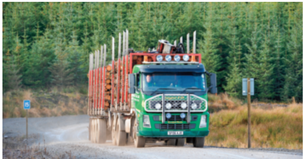
Timber lorry on a purpose-made unsealed timber haul road.
