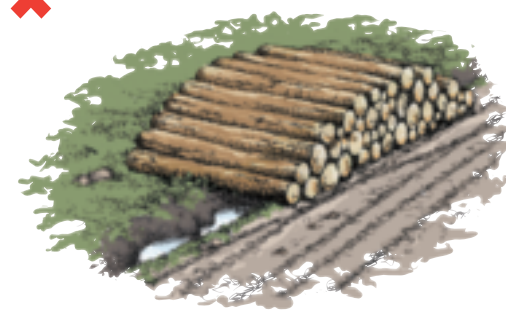
Logs stacked over ditch
