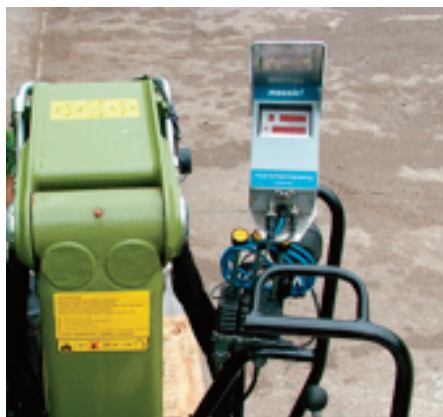
Load weighing devices may be fitted to lorry-mounted loaders.
