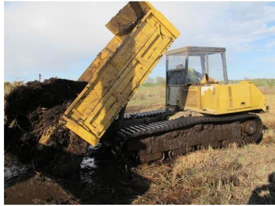
**Figure 20b.** Light-weight tracked dumper off-loading peat from peat cutting 1 at the outflow end of the bypass pipe, 13 May 2013.
