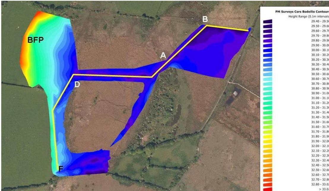
**Figure 11.** Topographic survey plot for the ditch network and surrounding peat surface in the western part of Cors Bodeilio NNR. Levels are shown as colour-coded 0.1 m height intervals. The yellow line with letter-coded points shows parts of the drainage network. Bodeilio Farm Pond is indicated as BFP.
