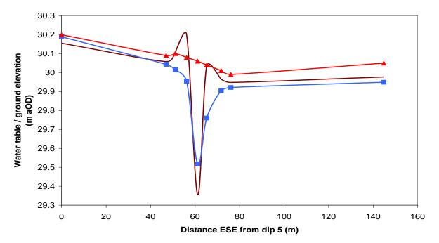
**Figure 8**. Variation in ground (brown) and water table level (blue, 24/11/11; red, 24/12/13)) for a 145 m levelled transect running WNW to ESE between dipwell 5 (SH 50053.77703) and dipwell 4 (SH 50178.77630). Ditch section A-B is crossed at c. 60 m. The blue and red plots show the respective water table profiles before and after infill of ditch section A-B; the brown line shows the original pre-restoration ground profile. See Figures 2 and 18 for transect location.
