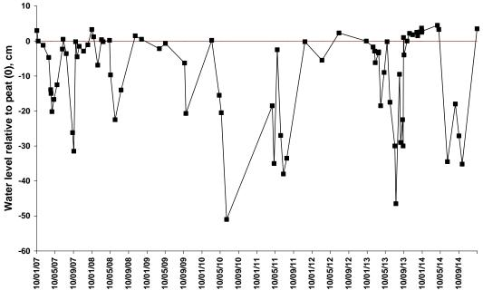
Figure 29. Manual dip record for dipwell T2-6.
