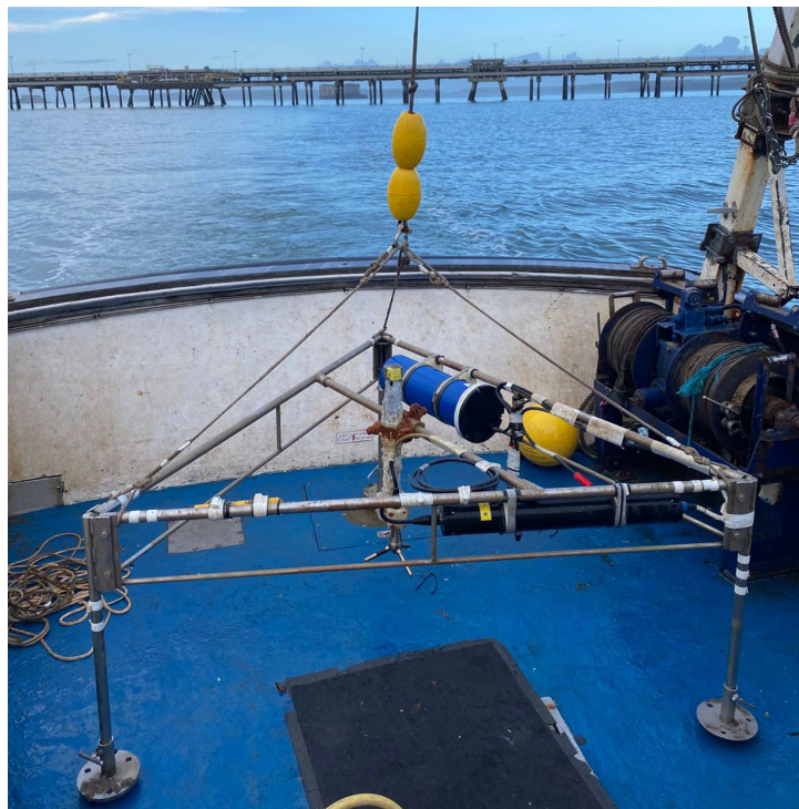
Figure 3. Instrument frame used to support the ADV and OBS sensors on the seabed. A surface marker buoy was attached to the frame for recovery and instrument visibility.
