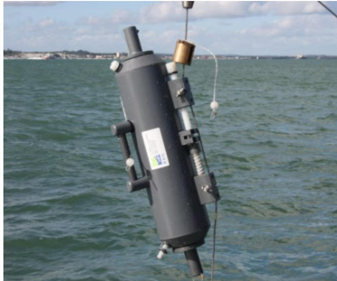
Figure 4. Niskin bottle used to collect sub-surface water samples from the area of the OBS sensors.
