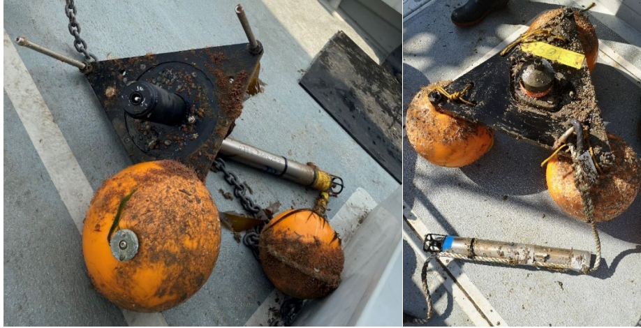
Figure 3. Left: Point Lynas inshore mooring recovered on August 10 th 2023 with two floats missing from the ARC mooring system. Right: Example mooring with floats tied to the structure as an extra securing measure.
