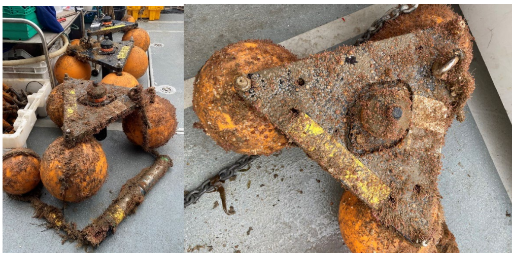
Figure 4. Left: Photographs of the three deployment moorings on August 10 th 2023. At the front of photo Point Lynas offshore, middle Holyhead deep and end Point Lynas inshore. Right: Close up photograph of the biofouling on the Point Lynas offshore mooring.
