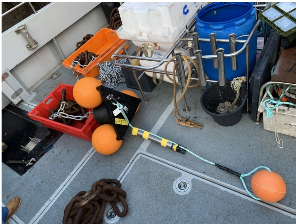
Figure 2. Example SoundTrap mooring. From left to right: 75kg chain clump, RS Aqua ARC canister and Vemco acoustic release, SoundTrap attached to line with submersible buoy for suspension above the seabed.
