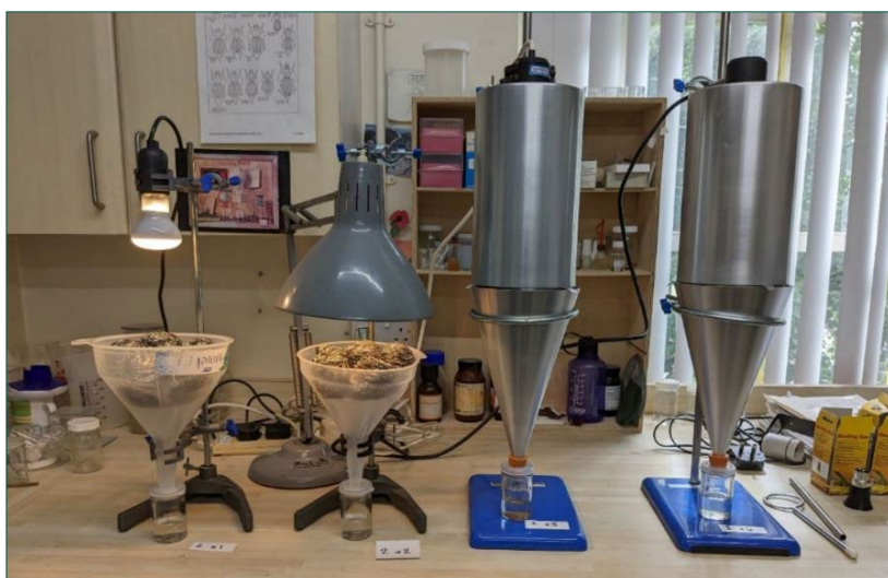
Figure 6. Tullgren funnel extraction setup.
