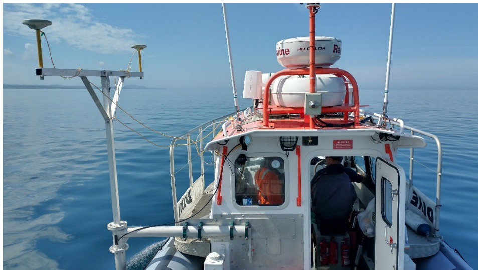
Figure 10: Survey pole and T-Bar in deployed position on Pedryn during multibeam echosounder survey of the Pen Llŷn A'r Sarnau Special Area of Conservation Modiolus modiolus reef and the additional reef area north of Porthdinllaen, in 2024.
