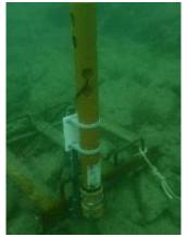
The greatly reduced seabed frame at Thorn Rock functioned perfectly well as a mount for the sediment trap (Newman Poot Collector – pat. pending) with new mounting arrangements made from recycled parts from the seabed settlement plate studies carried out in previous years.
