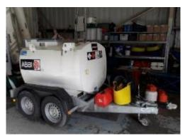
We do, however have a very shiny (albeit a cast off from another part of NRW) fuel bowser. This came with a powered pump, which makes fuel delivery to *Skalmey* at Martins Haven rather easier than the previous gravity powered system. The tank is double-skinned to prevent spillages and we carry a full spill kit if the worst should happen.
