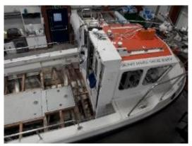
Skalmey has now served the MCZ (and MNR before that) for 27 years and so a thorough "health check" seemed in order. After a detailed professional survey of the hull and the equipment of the boat considerable remedial action was recommended. This included replacement of the deck and deck beams (now distinctly soggy and saggy in parts), replacement of windows (dribbly), replacement of the fuel tanks (crusty) and thorough overhaul of the engine (wheezy).
