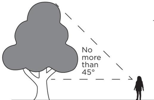
Figure 2. Correct distance from tree for hypsometer measurement.
